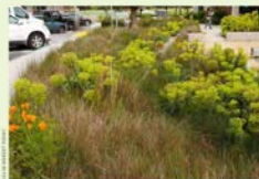
▲ This rain garden at the Sacramento Library front entrance accepts runoff from a large parking lot.
