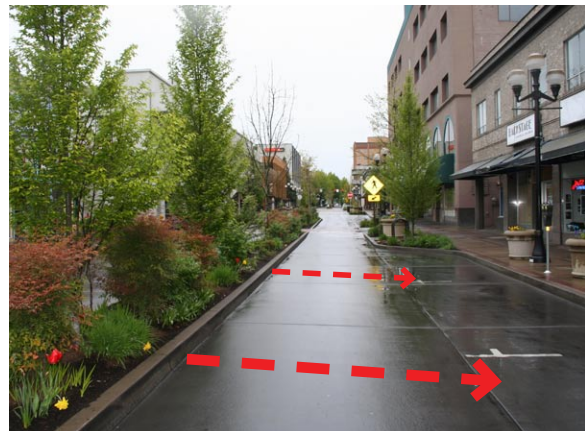
Figure 5-9: This crowned street has an existing landscape center median. Unfortunately, runoff cannot be easily routed to the center median because runoff is directed away from it.
