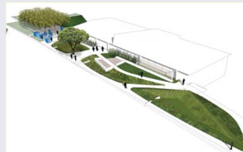
Scheduled for completion October 2009, the parking lot at Daly City's Serramonte Library will direct stormwater runoff through a series of vegetated detention swales/ponds for groundwater recharge.
